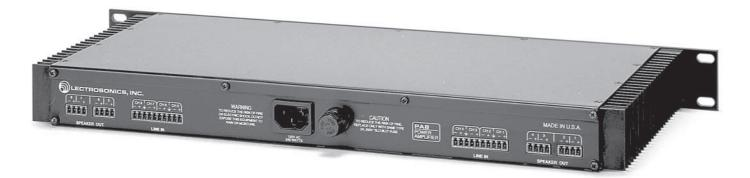
The PA8 8 Channel Power Amplifier is a unique single rack-space solution for zoned, distributed loudspeaker systems. The PA8 has eight separate power amplifiers, each with an output power capability of 10W (4 Ohms) or 6W (8 Ohms). The PA8 is passively cooled, and features full short-circuit and thermal overload protection. The amplifier outputs are muted at turn-on and turn-off, to eliminate transients.
